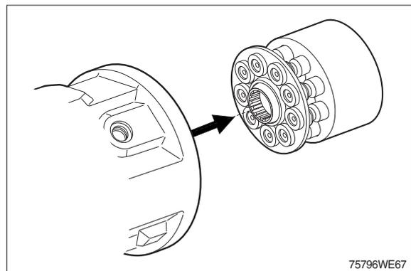
(6) Remove swash plate and bearing shells.
