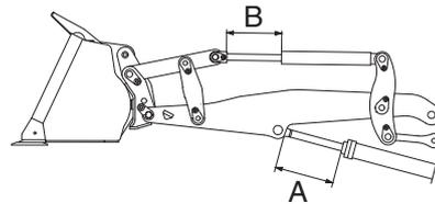
A : Retraction of boom cylinder rod
