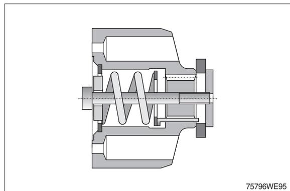
(5) Assemble piston with retaining plate.
